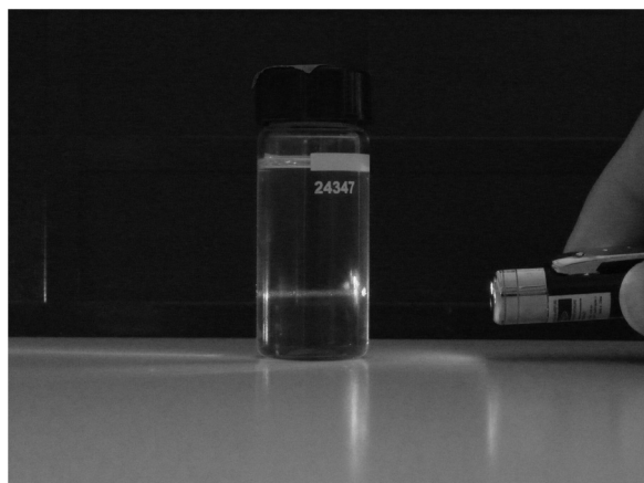
Fig. 5. Laser beam passing through a 1.5% (w) tetrabutylammonium alginate (TBA-Alg) dimethylformamide (DMF) solution with a turbidity of 4 NTU.
